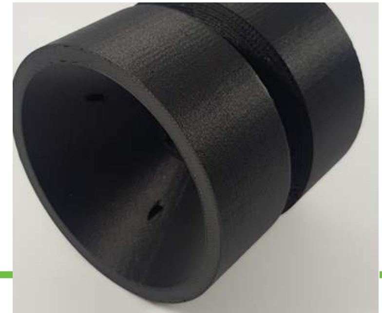
Printer: Fortus 450MC STRATASYS Material: Nylon12 CF
