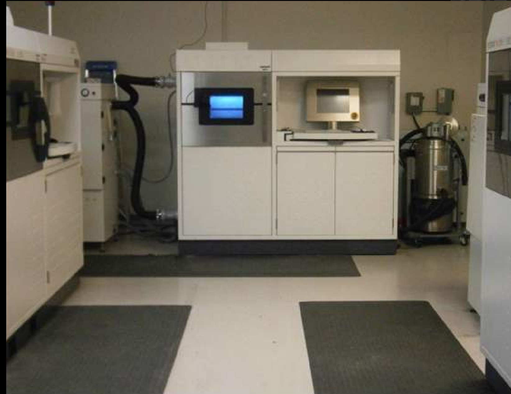
Explosion proof room, large outdoor argon gas tanks, 480V 3 phase, respirators, specialized operators, $600k printer + $200k post processing equip. + $200k facility
