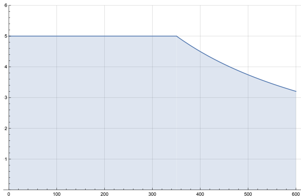
2.4: The relationship between the rated payload and the center of gravity offset.
